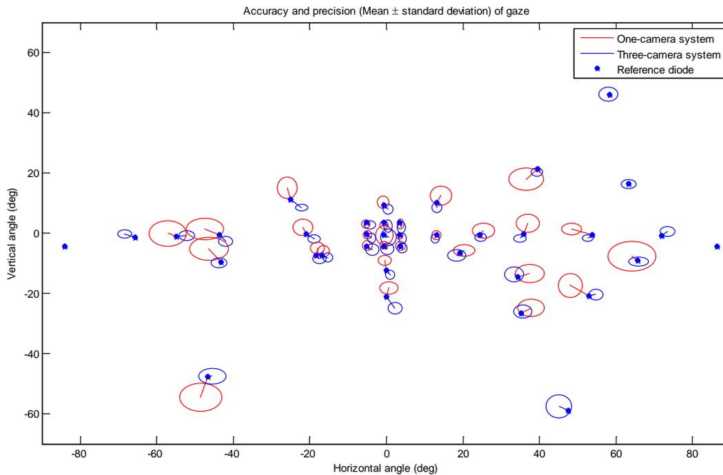
**Figure 4. Precision and accuracy of the measurements for each dot, where the ellipses indicate the average standard deviation across participants and the lines indicate the accuracy (distance from the reference point). Results are omitted in cases where the precision calculations are based on less than 15 % of the data.**
