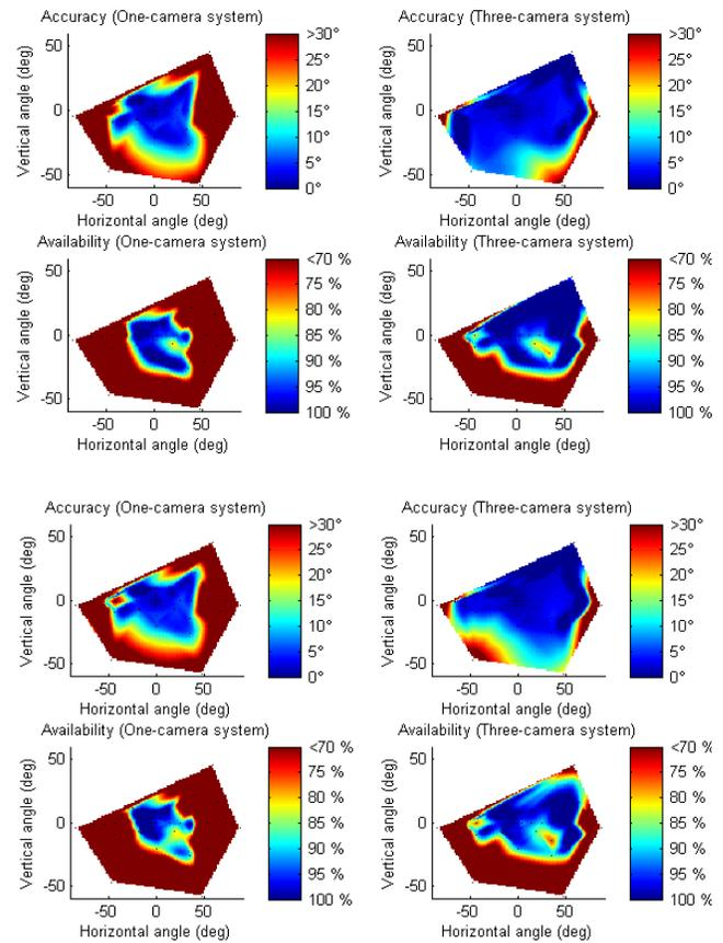
**Figure 3. 2D-maps of accuracy and availability encoded by color. The top four subplots illustrates when the participants are not wearing glasses and the bottom four subplots illustrates when they are wearing glasses.**
