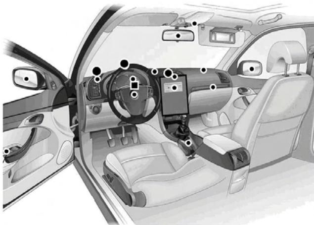
**Figure 1.** The layout of the LED inside the cockpit (small dots: LED; large dots: eye tracking camera location for three-camera system; square: eye tracking camera location for one-camera system).
