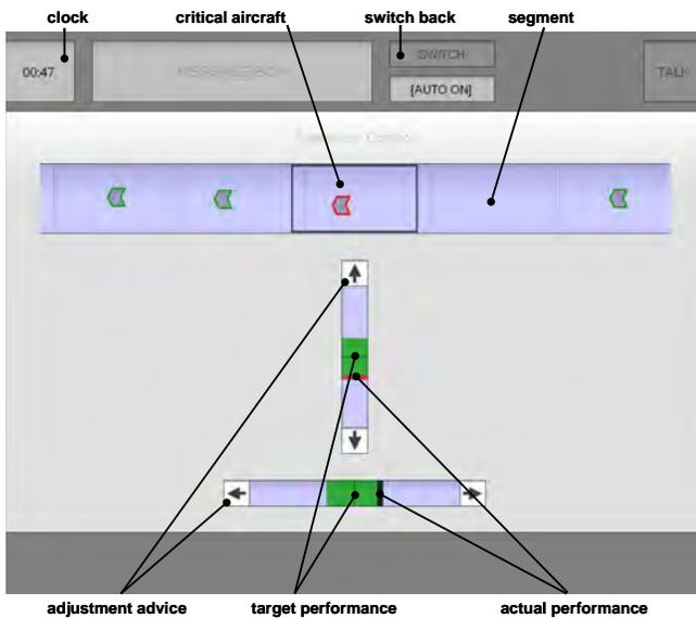
**Figure 3. Flight control display of the SSAS.**
