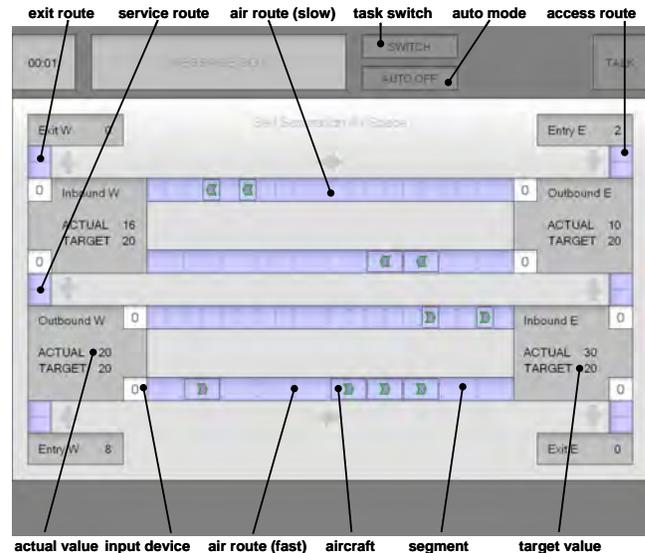
Figure 2. Air traffic flow display of the SSAS.
