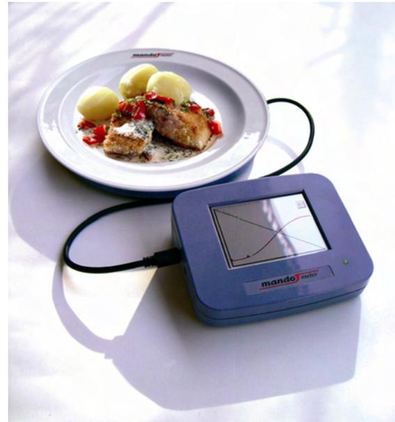
**Figure 1. The Mandometer<sup>®</sup>, a personal computer connected with a scale recording the meal in real-time. Feedback to the user can be provided through the touch screen.**
