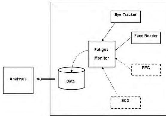
Figure 4. Fatigue monitor environment.
