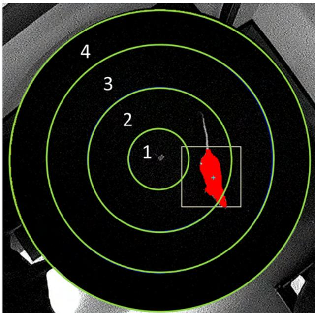
**Figure 1.** Top view of platform area showing the 4 circular sub-areas identified by the green lines, and the threshold image of a rat (red area). A white cross, that marks the centre of gravity in the threshold image, is taken as the actual position of the rat on the field.
