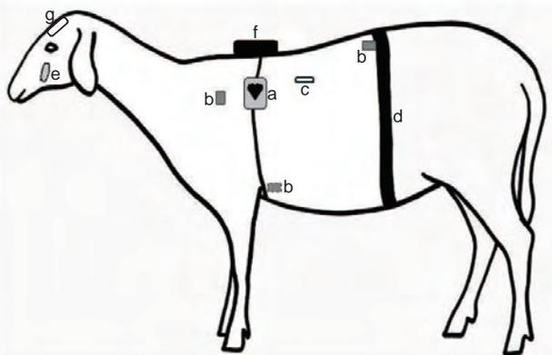
**Figure 1.** Sheep wearing measurement equipment (adapted from [7]): a) electrocardiogram holter and b) electrodes, c) electro-dermal activity device, d) respiration rate device, e) eye camera, f) battery pack, g) fNIRS sensor.
