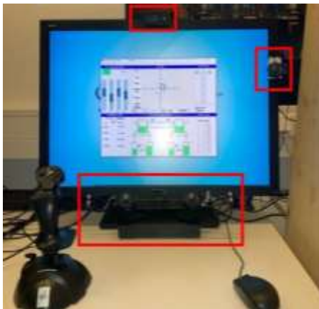
Figure 2. Experimental setup of the eye-tracker (top right and bottom center) and webcam (top center).
