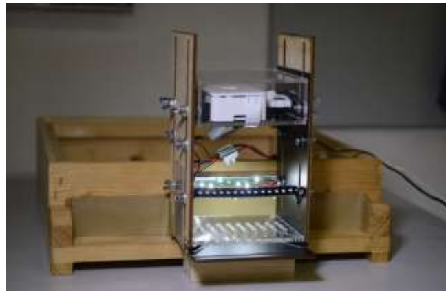
Fig. 1: A picture of the final prototype for bee mite monitoring. It is mounted at the entrance of a bee hive floor. The acrylic glass on the top protects the computing unit from rain. (Image from [10])
