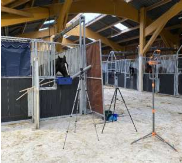
Figure 1: Experimental set-up with the feeder (blue box and grey pipe) attached outside the stable.
