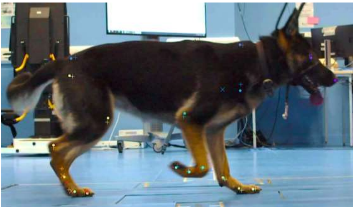
Figure 1 Diagram presenting validation methods of AI-based markerless tracking. The image depicts a snapshot of our bespoke convolutional neural networks estimated landmark locations from a lab-based gait trial on a domestic dog (German shepherd). Human-tracked landmark locations are denoted by the solid-coloured circles, and DLC landmarks are represented by the cross and plus symbols. The plus symbol represents DLC's landmark tracking when this surpassed the predetermined confidence threshold ( p > 0.6 ), with the cross-symbol highlighting tracking below this limit of confidence.
