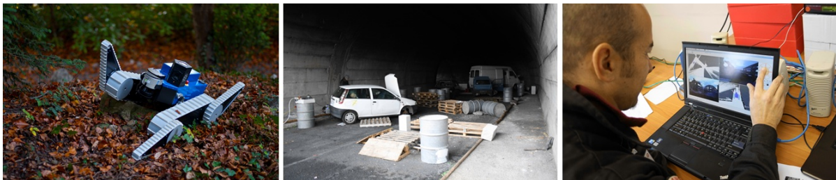
Figure 1. Left is a picture of the UGV, in the middle is a picture of the tunnel scenario on the right a participant is tele-operating the UGV.
