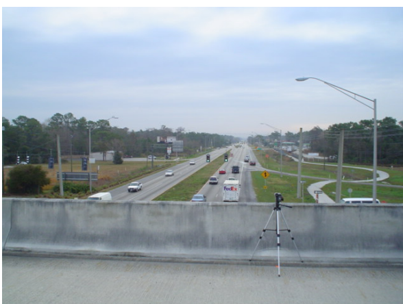
Figure 3. Video camera positioned on the bridge and road tubes placed every 100 feet along the arterial.
