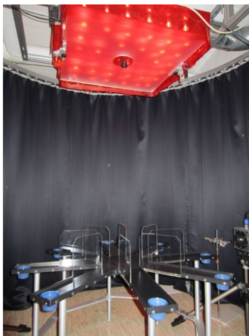
Figure 1. Setup for playback experiments and red light device. Elevated eight arm radial maze equipped with two ultrasonic microphones and two loudspeakers (Avisoft Bioacoustics; Berlin Germany). The rat's behavioral responses during playback of ultrasonic stimuli are recorded with a video camera positioned above the elevated eight arm radial maze. Testing is performed under dim red light.
