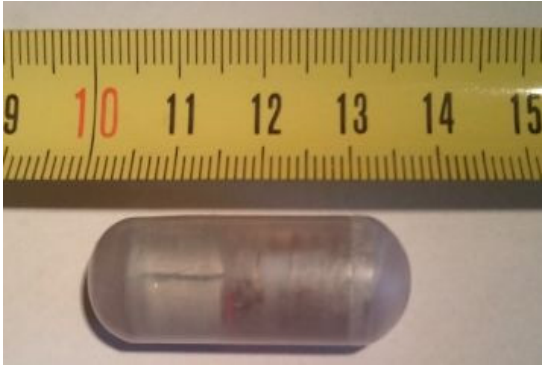
Figure 2. Encapsulated implant (SI ruler)..
