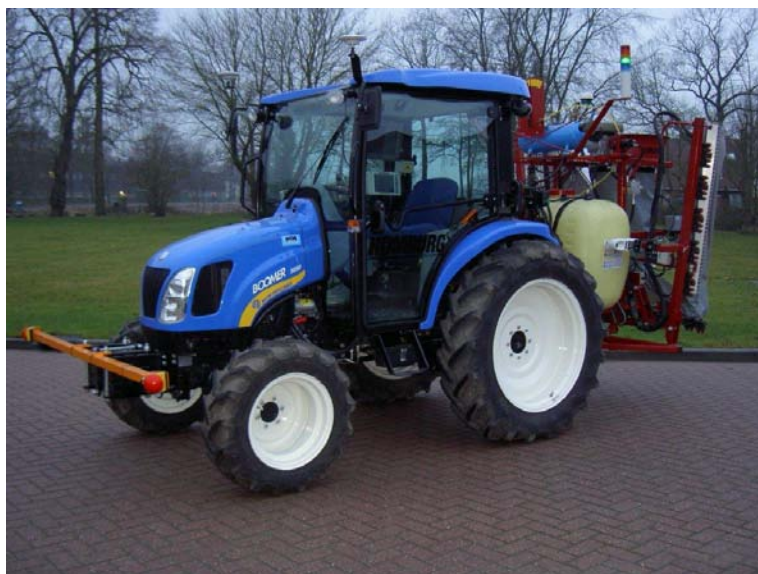
Figure 1. Autonomous tractor used to apply pesticides in strawberry fields. At present, the only safety feature of this tractor is the front-mounted bar with emergency stop buttons at either end.
