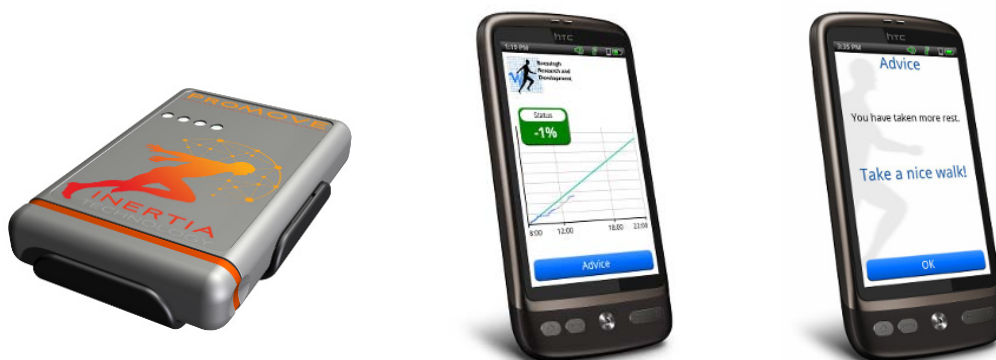
Figure 1. The Activity Monitoring and Feedback system from Roessingh Research and Development. Depicted is the ProMove-3D activity sensor, and two screenshots of the Smartphone interface showing a graph of daily activity and a motivational message.
