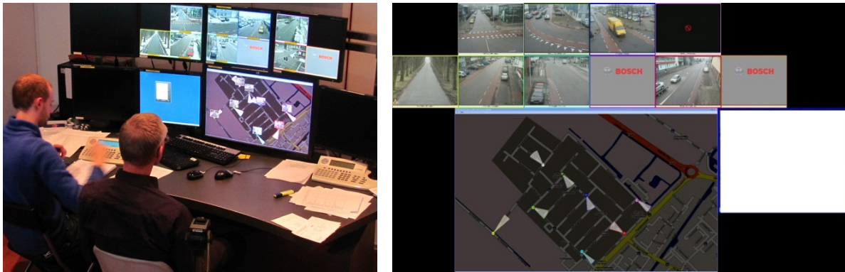
Figure 2. The interface (Left) centered on a map display showing color-coded camera viewing cones. The map display (Right) increases spatial awareness of the camera locations, orientations, and zoom. The color coding helps to match the image above to the viewing cone. Located at the CIV (Centrum voor Innovatie & Veiligheid) of the city of Utrecht.
