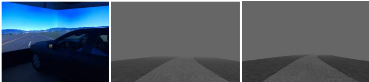
Figure 1. Left panel shows a picture of the driving simulator at the Hamilton Glaucoma Institute at UCSD. It provides a realistic driving experience with simulated vehicle motion and vibration, natural steering and pedal feel, and a 180 degree horizontal field of view plus rear and side mirror views. The provider is Realtime Technologies, Inc. ( http://www.simcreator.com/ ). The middle panel shows the experimentally used front scene image at 30m visibility and the right panel the 60m visibility. The contrast between the light lane and the darker ground surface was 25%.
