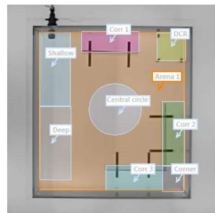
Figure 1. The MCSF arena with the different zones marked out.
