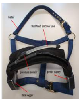
Technical components Pressure sensor, data logger, power supply
