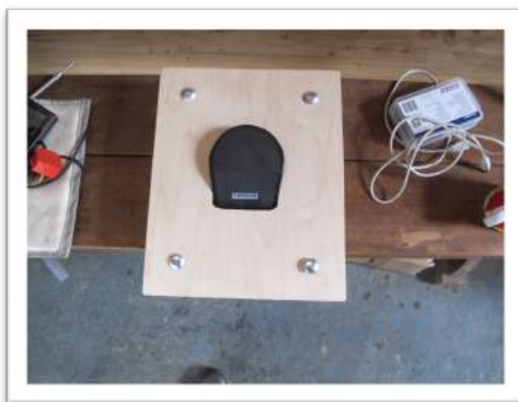
Figure 5: Button made from sewing machine pedal
