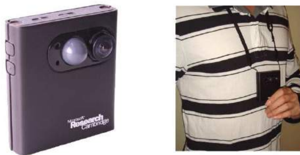
Fig. 1 The Microsoft SenseCam (right as worn by a user).
