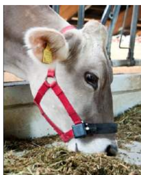
Noseband sensor Rumination, feed and water intake
