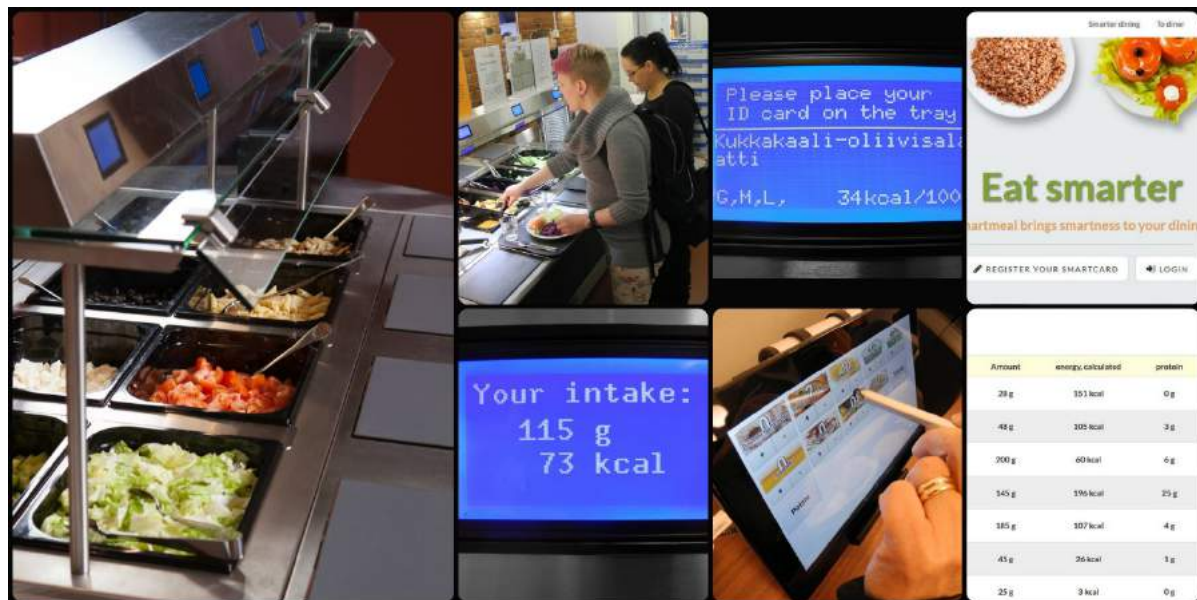
Figure 1. Description of Smartmeal: There is a Smartbuffet Unit with scales and embedded software integrated into the kitchen management software on the left. Smartbuffet Unit has displays which show the name of the dish, special diets and the amount of calories in 100 grams to all customers. Customers using Smartmeal have registered and they have a remotely readable rfid card to identify themselves. The displays guide identified customers to take their portion and indicate the amount of food taken and the calories in the portion. Food items such as drinks, bread, dressing and dessert are added with a touch screen application. The pictures on the right show that registered customers can see the summary of the meals and their dietary intake for a selected period on a webpage.
