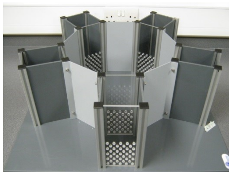
Figure 2. AGORA maze with an inside decagon and peripherally attached cubicles (Ugo Basile).
