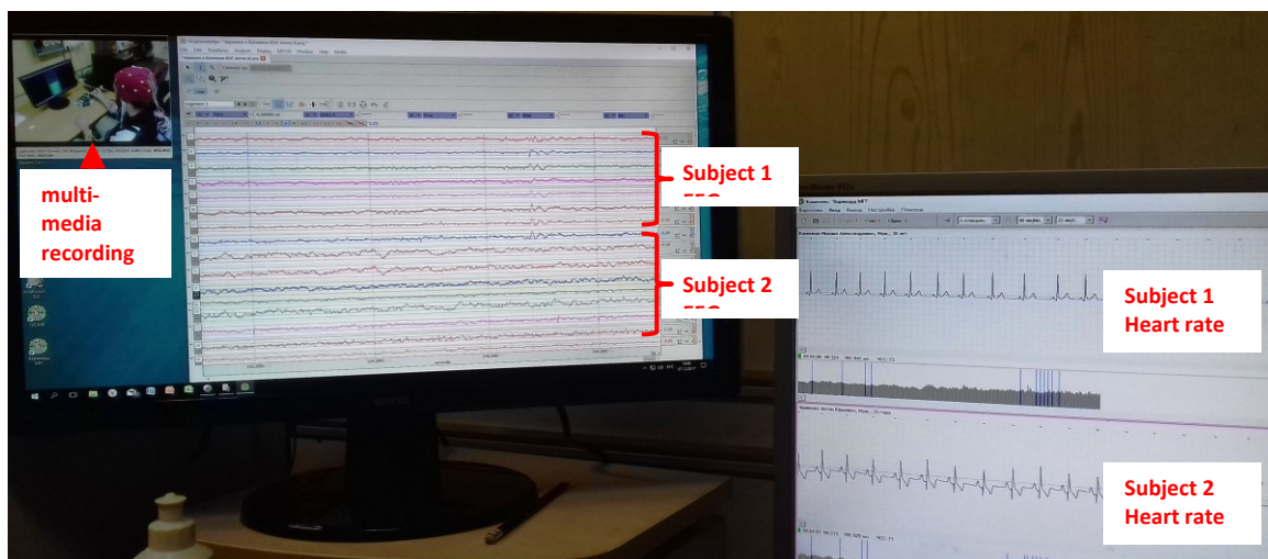
Figure 1. Illustration of the telemetry encephalograms and electrocardiograms recording in two participants.
